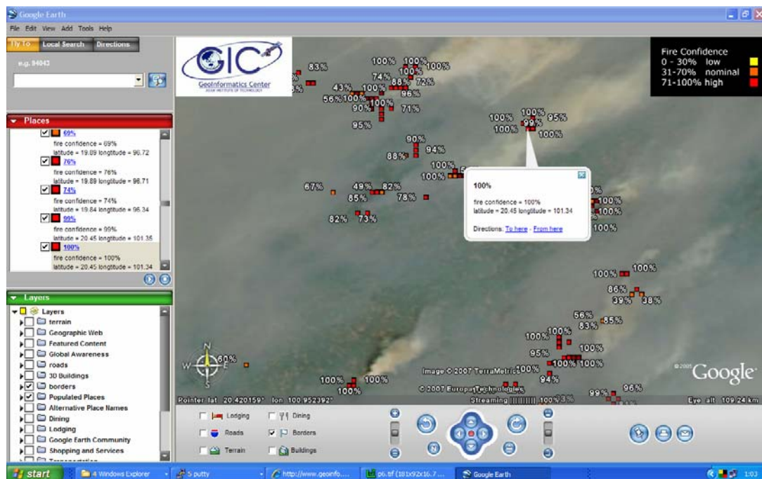
Figure 9 Visualization of the MODIS active fire pixels information on Google Earth 3D viewer of a specific area with Zoom-in mode. In this Figure, the strong smoke and its fire location is shown
